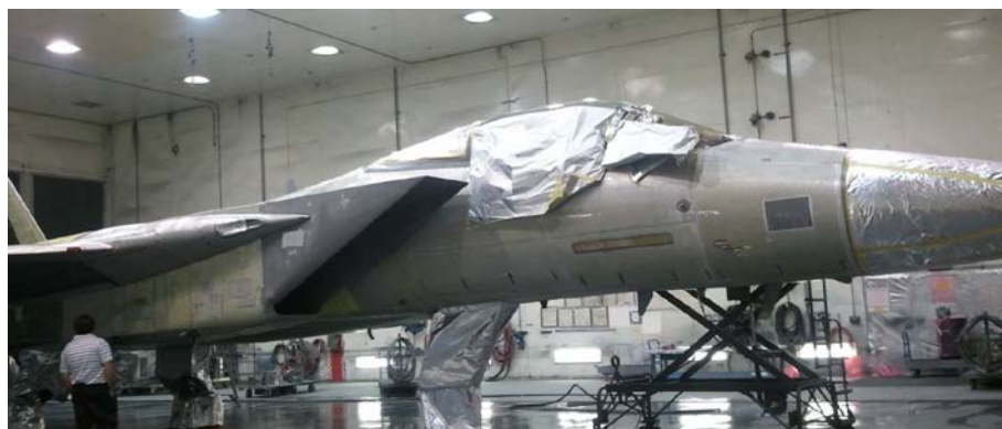
Figure 10. F-15 with Deft Rare Earth Cr-free paint system.
