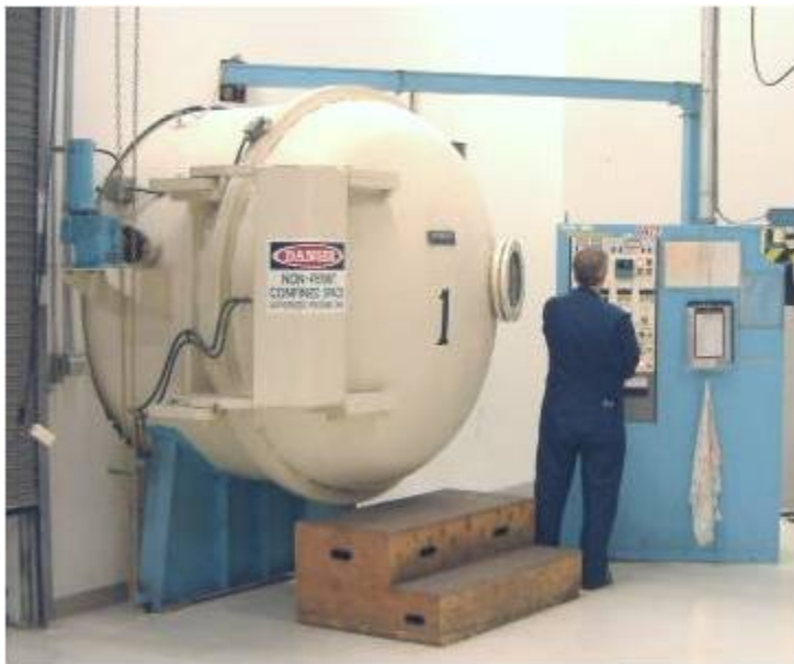
Chamber for IVD aluminum (also known as an Ivadizer)
