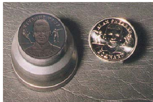
Figure 5. MoST-coated coining die (Courtesy Teer Coatings)
